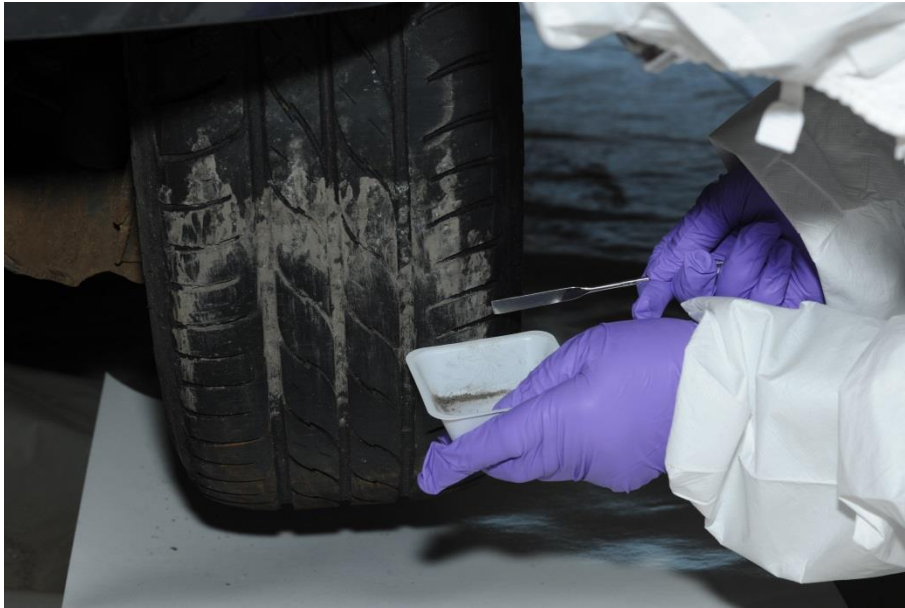
Figure 8. Use of a sampling boat to collect discrete samples (in this case where a tyre had been sitting while the rest of the vehicle had been jet washed).
